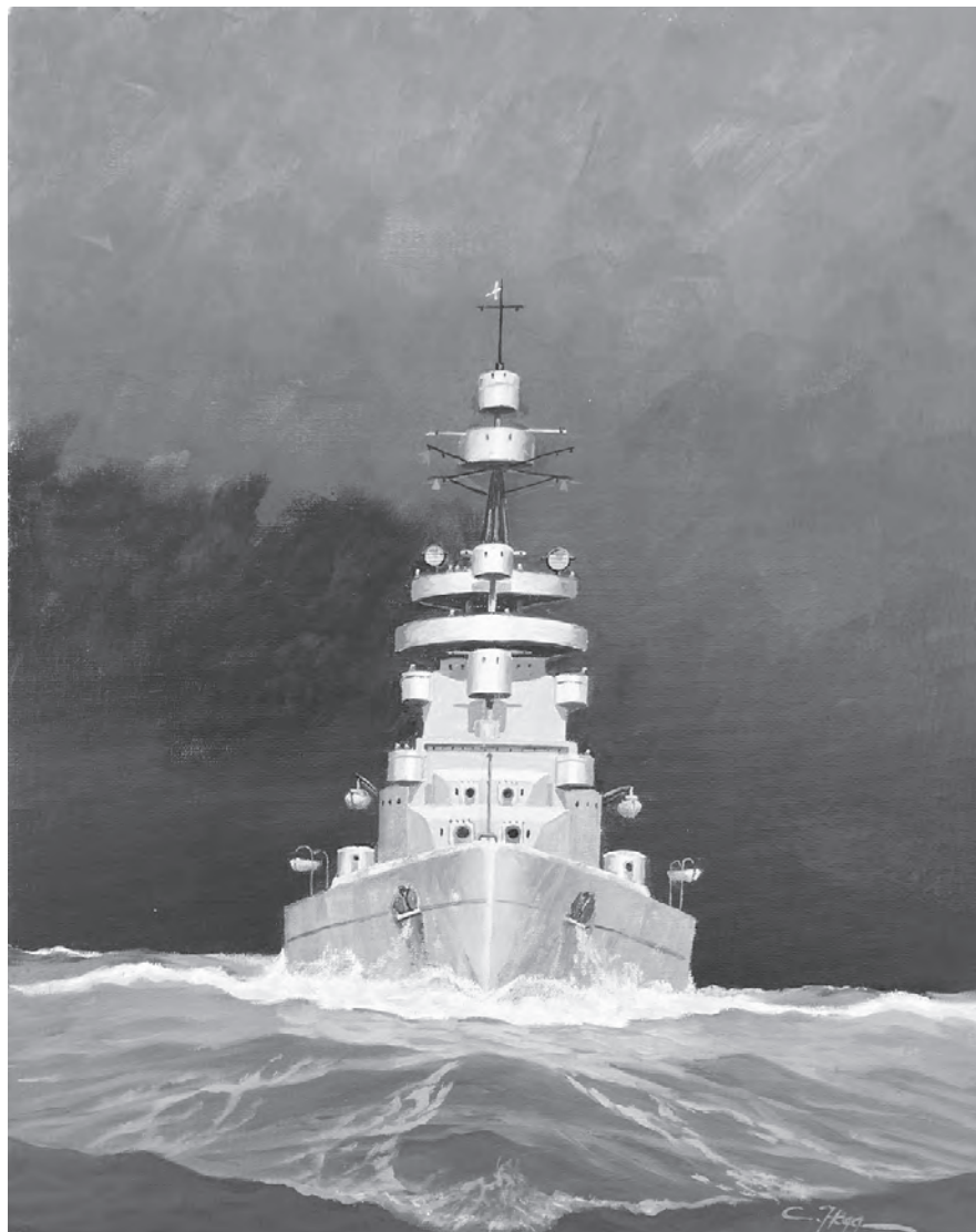
The late 19 th /early 20 th century modernisation of the Swedish Navy was exemplified by the coast defence ship HSwMS Sverige, 1915-1953. 7,600 tons. 4 x 11", 8 x 6", 2 x 18" torpedoes. The government suspended funding after keel laying, but she was paid for by voluntary public subscription. Paraphrase painting by Christer Hägg after a British original.
