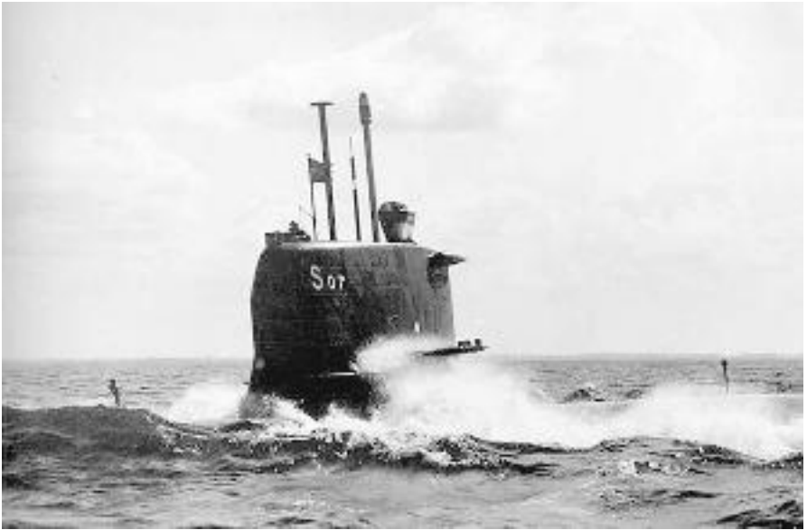
HMS Sjöormen at sea. The HF transmitting antenna is the mast with the horizontal disc; the VLF receiving antenna radome is at the top of the conning tower, aft. (Foto: Kockums)
